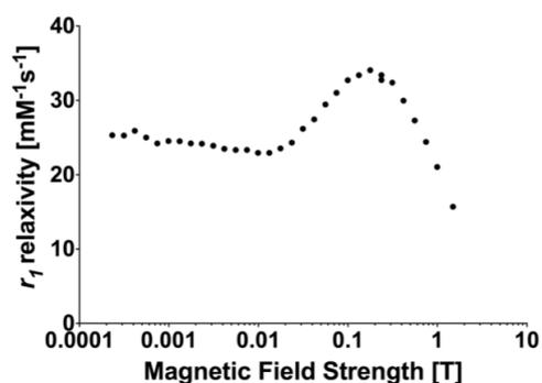
**Fig. 1.** Proton nuclear magnetic relaxation dispersion of Ferumoxytol (Feraheme) measured at 37°C.
