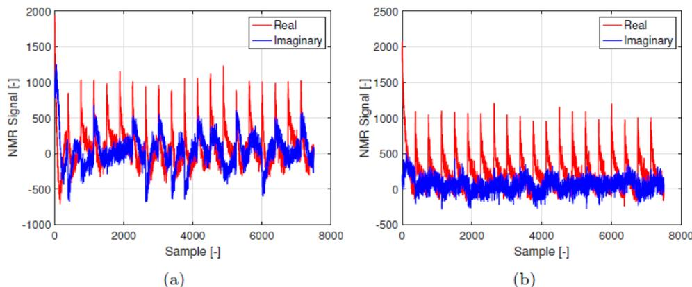
**Fig. 1.** FFC NMR experiment without lock system (a) and with lock system (b), in presence of a 10 Hz sinusoidal current disturbance.
