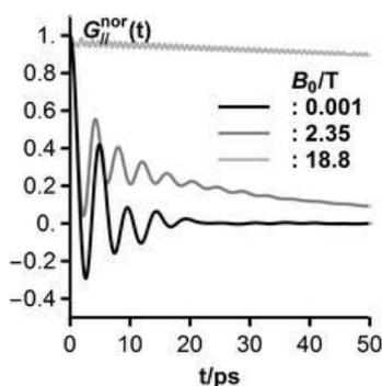
**Fig. 1.** Longitudinal relaxation function  $G_{ii}^{nor}(t) = \langle S_z(t)S_z \rangle / \langle S_z(0)S_z \rangle$  of an electronic spin  $S = 1$  with static and transient ZFS parameters  $\Delta_S = 5 \text{ cm}^{-1}$ ,  $\Delta_T = 2 \text{ cm}^{-1}$ , rotational and vibrational correlation times  $\tau_R = 100 \text{ ps}$ ,  $\tau_v = 5 \text{ ps}$  [3].
