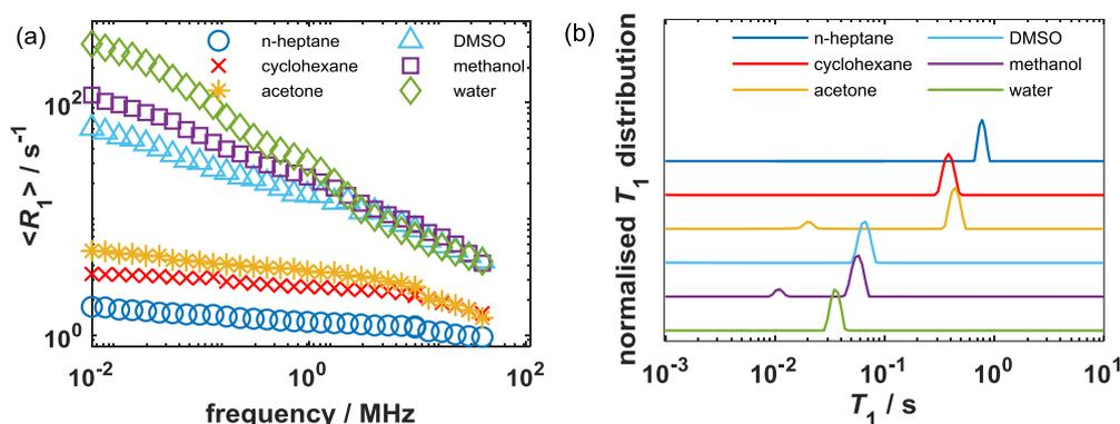
Fig. 1. The (a) NMRD profiles of six different liquids imbibed within  $\gamma$ -alumina and (b) the corresponding  $T_1$  distributions obtained at 1 MHz for each liquid.
