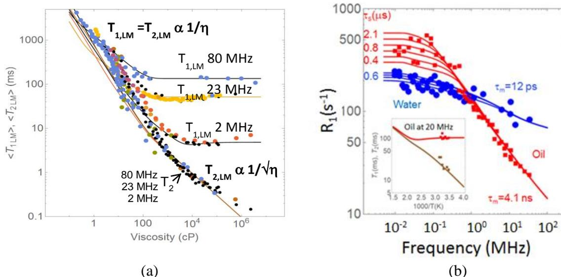
**Fig. 1.** (a) Comparison experiments-theory of the viscosity dependencies of several heavy crude oils. (b) Comparison experiments-theory of the NMRD profiles of brine (blue) and oil (red) in as received shale rock at room temperature. In inset are given the temperature dependencies of  $T_1$  (red) and  $T_2$  (brown) of oil in shale rock.
