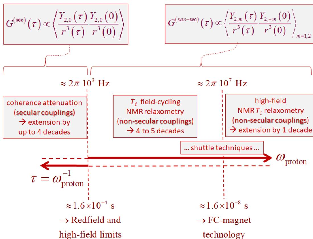
Fig. 1. Secular and non-secular dipolar correlation functions and the time and frequency scales to be probed by respective NMR techniques [1].
