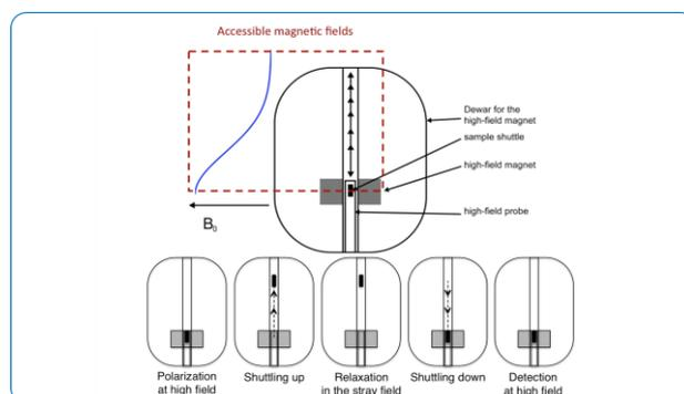
**Fig. 1.** Principle of high-resolution relaxometry.
