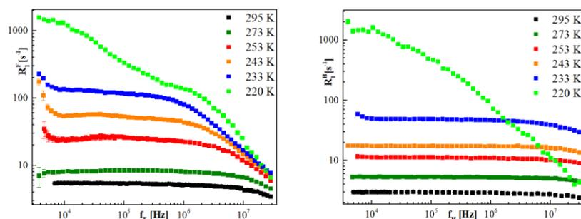
**Fig. 1.** NMRD profiles of C<sub>2</sub>F<sub>6</sub>LiNO<sub>4</sub>S<sub>2</sub> aqueous solution acquired at different temperatures for the <sup>1</sup>H and <sup>19</sup>F nuclei.
