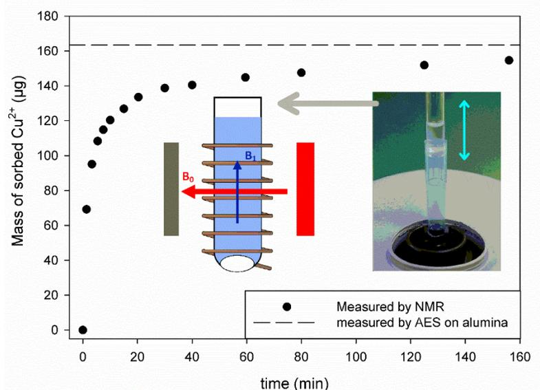
Fig. 1. Principle of the adsorption follow-up by NMR relaxometry
