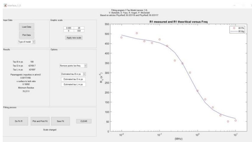
**Fig. 1.** Screenshot of the interface of the Matlab script 3τM. Measured  $R_1$  relaxation rates (open circles) for pure C<sub>3</sub>S hydrated, after one month hardening are plotted along with the fitted curve (continuous line).
