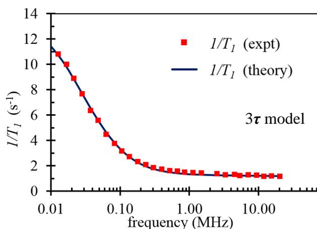
**Fig. 1.** The spin-lattice relaxation rate  $T_1^{-1}$  is presented as a function of frequency for a plaster paste sample from [3]. The solid line is the fit based on the  $3\tau$  model.
